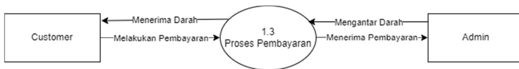
Gambar 10. Data Flow Diagram Level 1 Proses 3
